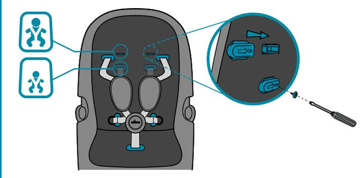
Use the harness fixing screws to secure the harness attachments.
