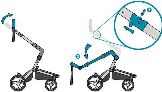
Rotate the handlebar into position 4. Push the safety button down, then pull the 2 folding locks upwards, then lower the handlebar section down.
